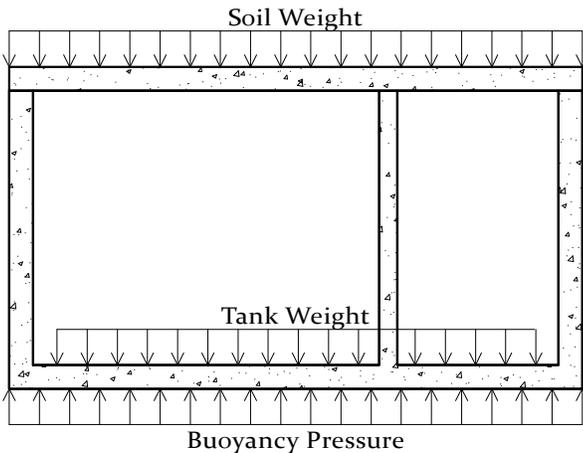
Yes indeed, concrete tanks can float! The following assumptions are made in determining the water level at which flotation occurs:
